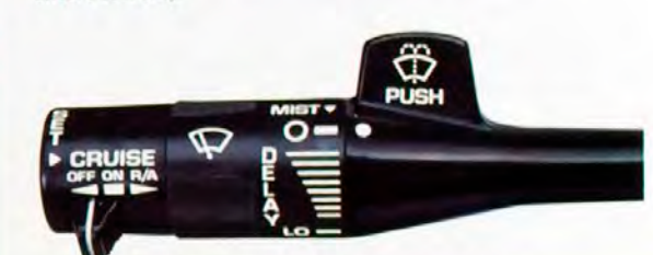
Optional electronic speed control and intermittent wipers are on the standard multi-function lever.
