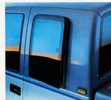
Extended Cab swing-out side windows.
