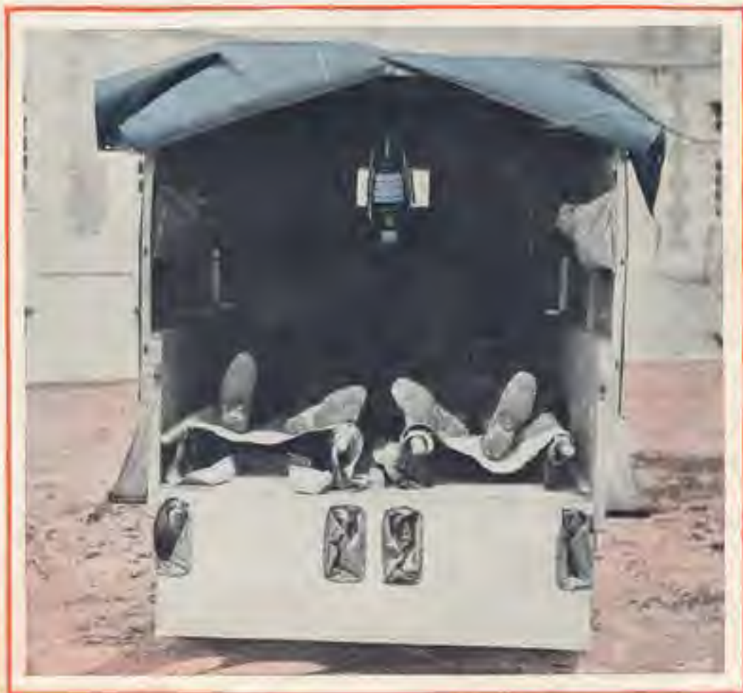
Showing how wounded soldiers are carried on army stretchers. Note pockets in tail board to receive the ends of the stretcher
