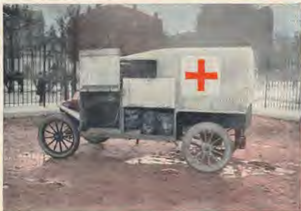
Ford supply and repair car showing some of the cupboards open
