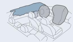
**FRONT, SIDE AND CURTAIN AIR BAGS** An intelligent front air bag system senses driver's seat position and front-passenger seat occupancy to determine the safest deployment level for each. And side-curtain air bags help protect front and outboard rear seat passengers.
