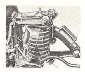
Heavy-duty front springs, heavyduty shock absorbers give longer life. Heavy-duty variable-rate rear springs (with 6 leaves), heavyduty diagonally mounted rear shock absorbers.
