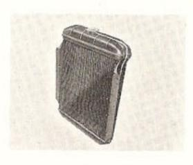
Specially designed heavy-duty Ford radiator has larger frontal area plus extra-cooling fan for improved cooling under extreme operation and temperature conditions. (Std. with Interceptor Y-8.)
