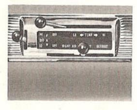
Ford's MagicAire Heating-Ventilation system controls heat distribution for warmth and defrosting, reduces window fogging. Recirculating type heater-defroster also available.
