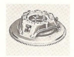
Heavy-duty 11" dia. clutch with ball-type release bearing having fitting for pressure lubrication built to take hard-wearing effects of rugged driving. (Standard with Interceptor Y-8.)
