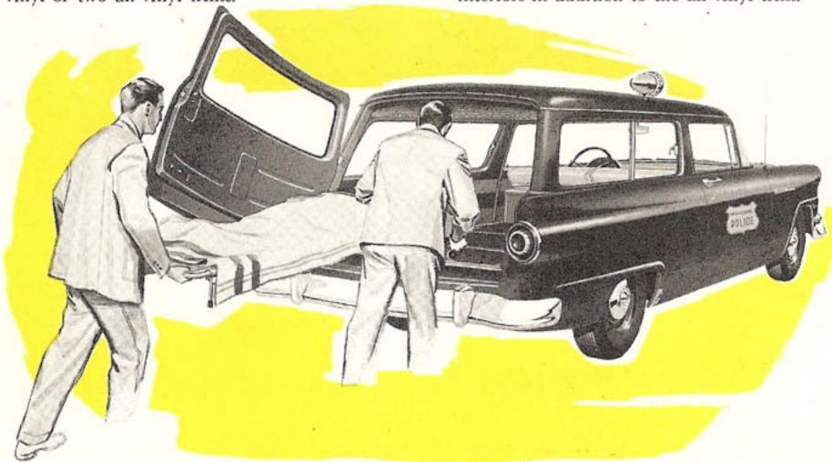
Ford Station Wagons may be ordered with a wide-opening panel-type door which stays open in all positions, or the standard tail gate which locks securely in either "down" or "up" position.
