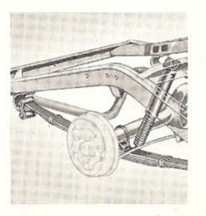
VARIABLE-RATE REAR SUSPEN-SION with long rear springs and tension-type shackles gives smooth, easy action over small road bumps, controlled action over big bumps. Starting and stopping are smoother too, because Ford's Hotchkiss drive uses rear springs to cushion severe braking and accelerating forces.
