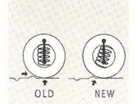
"floats" your passengers over rough roads! Springs are tilted to absorb road shock from the front as well as straight up and down. This gives passengers and driver a feather-soft ride—even reduces the little bumps they receive on paved roads, and makes the ride smoother on any road.
