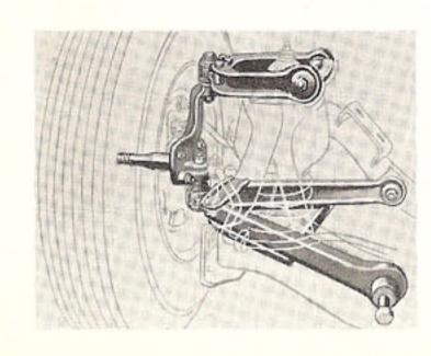
BALL-JOINT SUSPENSION, the most modern front suspension available, provides effortless handling on any type road! Wheel movement—up-and-down, left or right—centers around ball joints that can't bind or get out of line. Forged steel parts and resilient rubber bushings require less maintenance.
