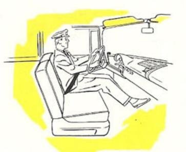
NEW FORD SEAT BELTS. These new seat belts, designed to exceed the rigid CAA requirements for aircraft, are the finest car seat belts available today. These safety items, available at extra cost for all models, front and rear, are made of strong nylon-rayon cord with buckles of die-cast aluminum quickly operated in one-hand release or adjustment. Each belt is securely anchored to husky steel plates reinforcing the steel floor structure.
