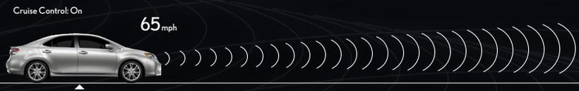
As you approach a slower moving vehicle in your lane, the available Dynamic Radar Cruise Control<sup>26</sup> automatically brakes to help you maintain a pre-set distance. Should the vehicle ahead change lanes, the system automatically accelerates until you've resumed your desired speed.
