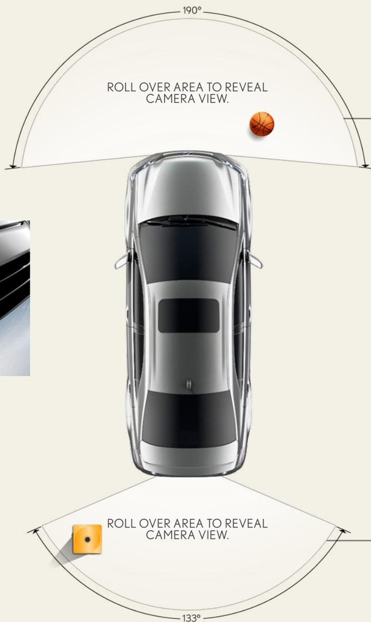
Using a specially designed wide-angle lens to help reveal hard-to-see areas, an available Wide-view Front Monitor<sup>6</sup> comes on at the touch of a button (or automatically, if you choose) when you're driving at low speeds. A camera mounted in the grille displays a 190-degree front view on the navigation screen.
