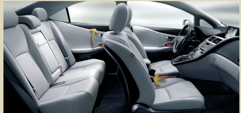
In certain low-speed rear-end collisions, active front headrests<sup>27</sup> raise upward and forward, helping to reduce the severity of a whiplash injury.
