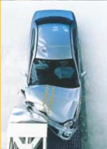
Ring-Shaped Reinforcement Frames in the front, center and rear of the body structure disperse impact energy around the passenger compartment, offering added protection for occupants. The center ring connects the center pillar with the lateral roof and floor supports for increased side-impact protection. In addition, a specially designed front sub-frame increases energy absorption in offset frontal collisions.
