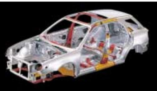
Careful computer analysis and design provides a structure that's stronger and more rigid than the previous Impreza. Front and rear crumple zones help manage impact energy by compressing at a controlled rate.
