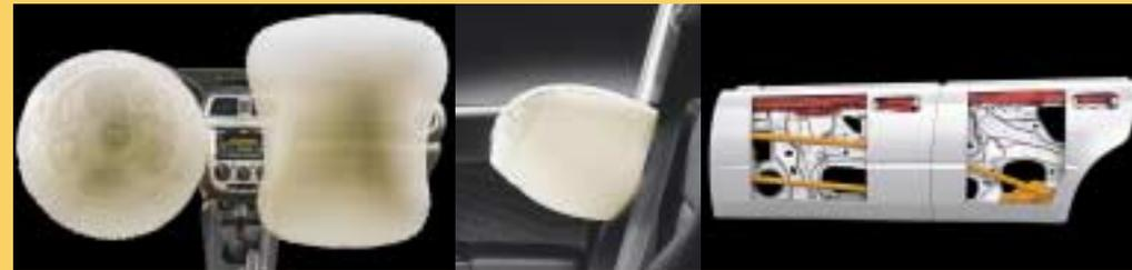
WRX models add standard front seat side-impact air bags. Mounted on the front seats, they maintain optimal placement regardless of seating position.\*
