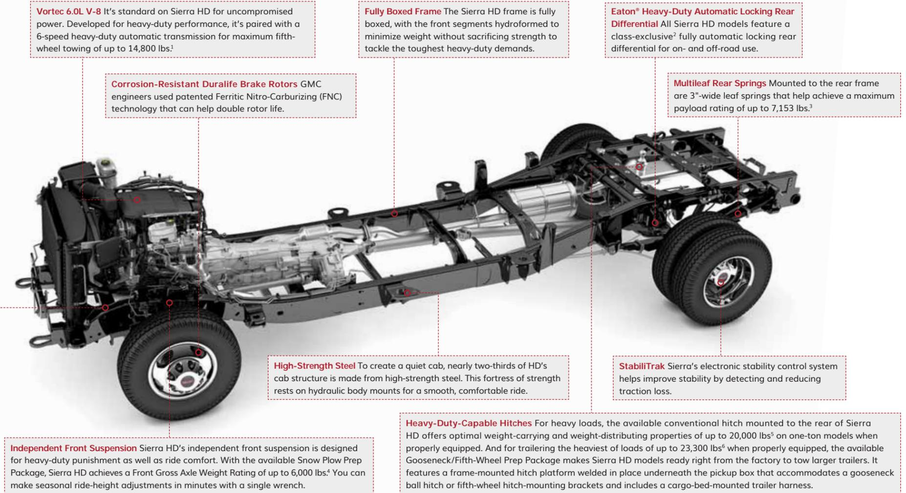
**Vortec 6.0L V-8** It's standard on Sierra HD for uncompromised power. Developed for heavy-duty performance, it's paired with a 6-speed heavy-duty automatic transmission for maximum fifth-wheel towing of up to 14,800 lbs.<sup>1</sup>
