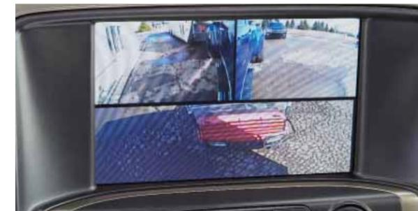
**Trailing Camera System-Associated Accessories** This available dealer-installed accessory system,<sup>2</sup> produced by EchoMaster, provides several vantage points for confident trailering. The system offers multiple simultaneous views around Sierra HD, including views from left and right side-view mirror cameras and a trailer-mounted camera.
