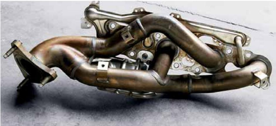
**4 INTO 2 INTO 1 TUBULAR EXHAUST MANIFOLD**
