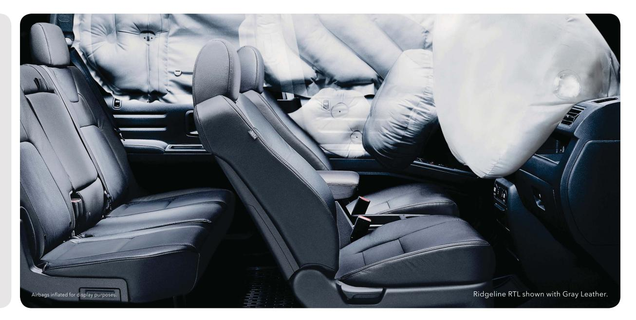
Front, front side, and side curtain airbags are all standard. The front seats feature active head restraints that are designed to move up and forward in a rear collision to help reduce the likelihood of neck injury.\*
