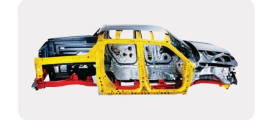
The Ridgeline's first line of defense is a reinforced unit body that incorporates a closed-box frame with internal high-strength steel frame stiffeners. Both the frame rails and all seven crossmembers feature box-section construction. The result is a remarkably high torsional rigidity.
