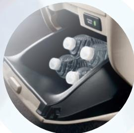
For refreshment, reach inside the new cool box. Located in the lower part of the center stack, it uses the A/C system to keep contents chilled (EX-L and above).
