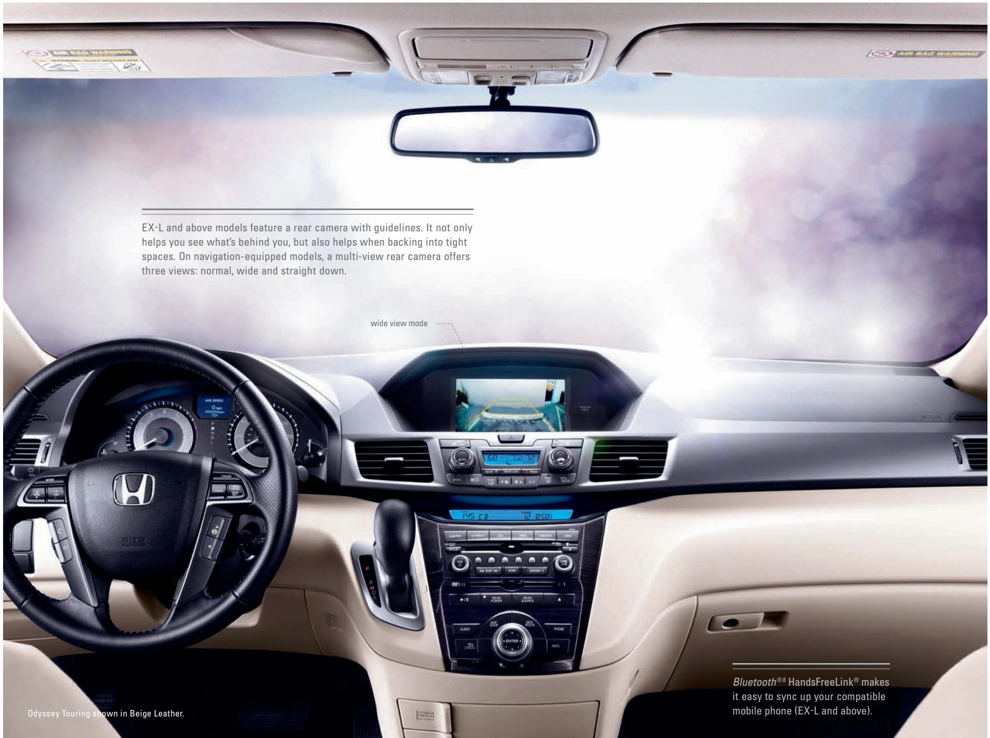
EX-L and above models feature a rear camera with guidelines. It not only helps you see what's behind you, but also helps when backing into tight spaces. On navigation-equipped models, a multi-view rear camera offers three views: normal, wide and straight down.
