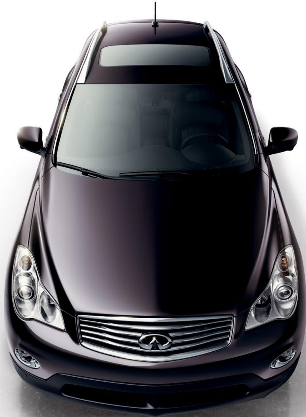
**INNATELY RESPONSIVE BALANCE** The engineering philosophy behind Infiniti performance sedans, the Front-Midship Platform, also underlies the design of the QX50. Placing the engine's center of mass just behind the front wheel center line creates a near-equal front-to-rear weight ratio, with a slight front bias that you'll feel as quicker turn-in and even balance as you accelerate out of a corner.
