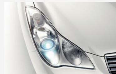
**A SMARTER WAY TO SEE** The Adaptive Front lighting System<sup>1</sup> on the QX50 lights not just the way ahead, but around as well. It directs light toward corners by turning the headlights in coordination with steering input to help the driver see upcoming vehicles and pedestrians, and to help you reach your destination safely.
