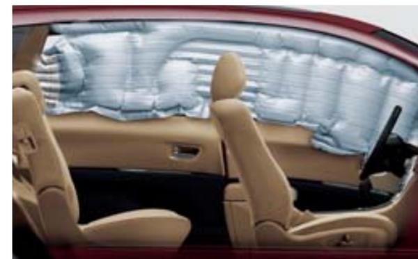
**Front, side and curtain air bags** An intelligent front air bag system senses driver's seat position and front-passenger seat occupancy to determine the safest deployment level for each. Front side-impact air bags are mounted to the seat to stay in position as the seat is adjusted. And side-curtain air bags help protect front and outboard 2nd-row passengers.
