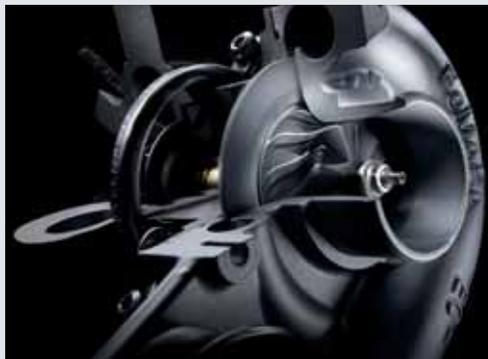
**TWIN TURBOCHARGERS** create exceptional power by recycling exhaust gas through turbines – spinning up to 205,000 rpm – to pressurize or “boost” the air that mixes with atomized fuel in the combustion chamber. The turbo’s convection cooling system works even after the engine is turned off, to help eliminate the extreme-heat issue of coking. And performance is unaffected in high-altitude environments.
